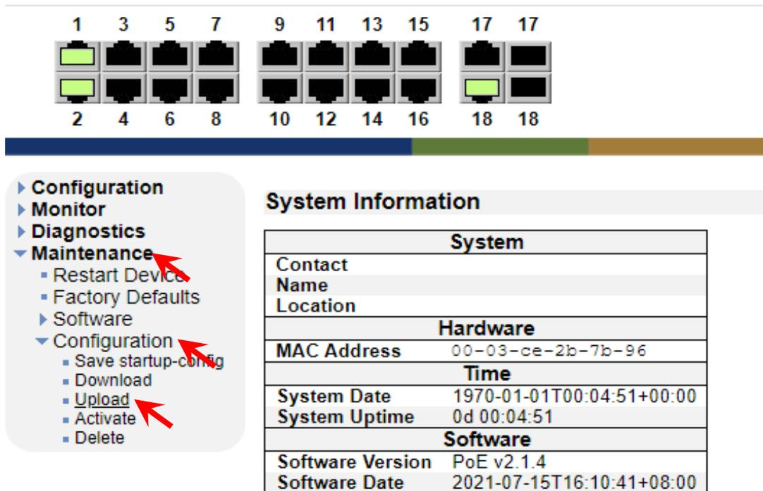
The image shows a network switch with 18 ports arranged in two rows of nine. Ports 1, 2, 17, and 18 are illuminated with green lights. Below the switch is a navigation menu with 'Maintenance' selected, and 'Configuration' > 'Upload' highlighted with red arrows. To the right is the 'System Information' page with the following data:
