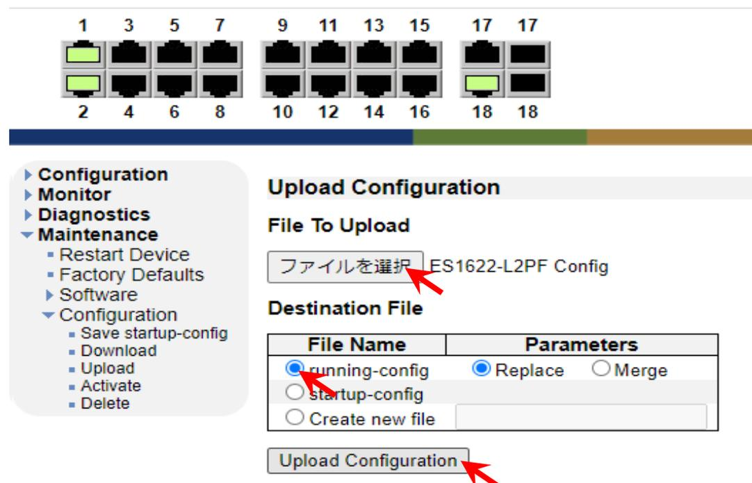
The image shows the same network switch as above. Below it is the 'Upload Configuration' page. The 'File To Upload' field contains 'ES1622-L2PF Config' with a red arrow pointing to the 'ファイルを選択' button. The 'Destination File' section has 'running-config' selected with a radio button, and 'Replace' selected with a radio button. The 'Upload Configuration' button at the bottom is also highlighted with a red arrow.
